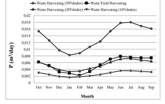
Fig. 5. Comparison diagram of monthly harvested water in the field method with theoretical indices  $(m^3/day)$
