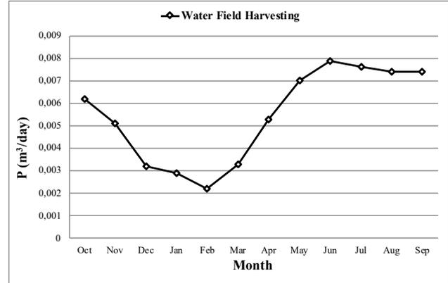
Fig. 4. Diagram of monthly harvested water from screen collector device ( $m^3/day$ ).
