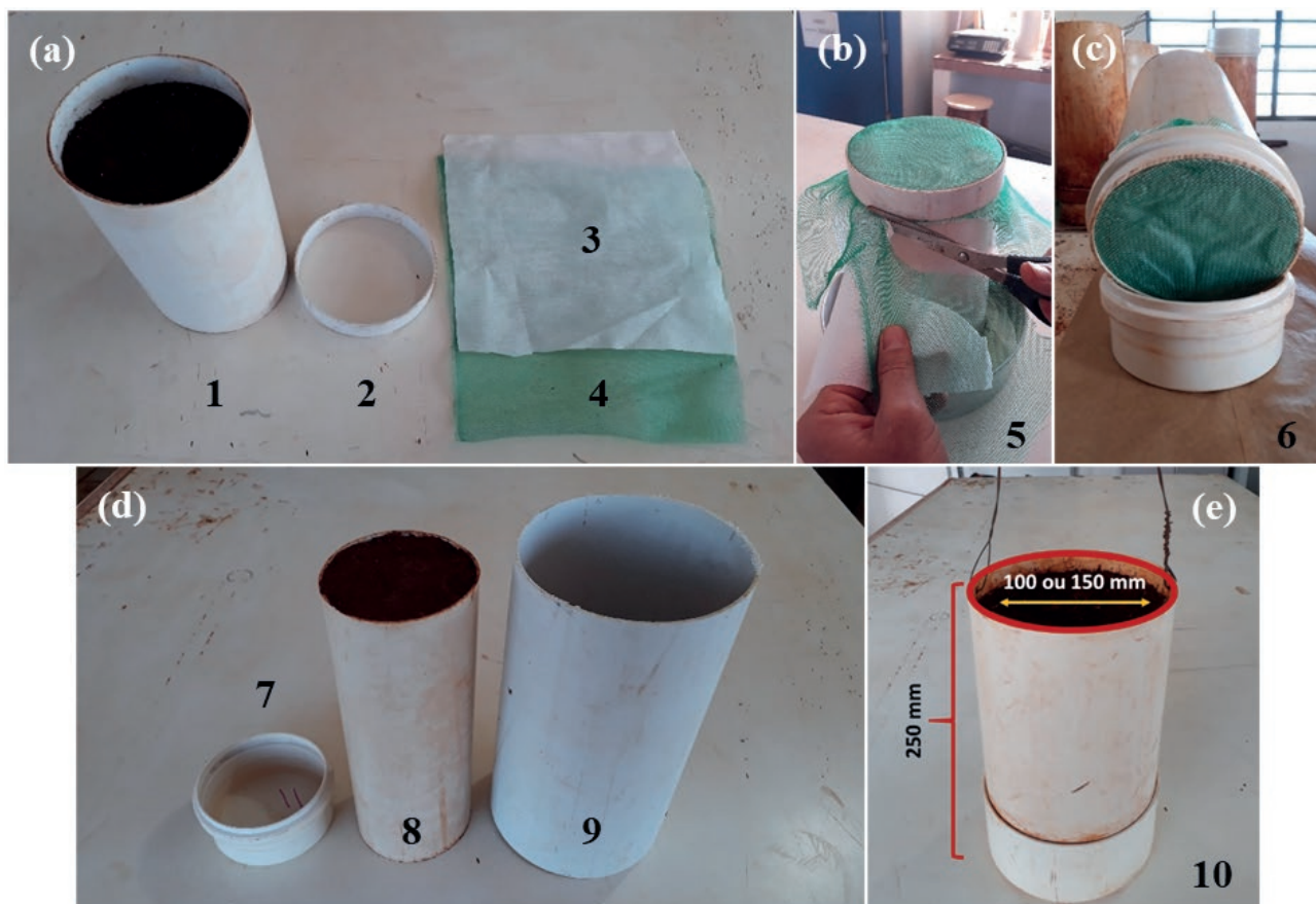
Fig. 3. Open-bottom microlysimeter model with water drainage (A, B and C); Microlysimeter model with closed bottom without water drainage (D and E). 1 - Internal structure; 2 - Open CAP; 3 - 80 gram white TNT (30 x 30 cm); 4 - 0.1 mm nylon mesh (30 x 30 cm); 5 - Mounting the TNT, the nylon mesh and the CAP on the internal structure; 6 - Bottom of the internal structure of the microlysimeter after it is ready; 7 - PVC closed cap; 8 - Internal structure; 9 - External structure; 10 - Microlysimeter with closed bottom.
