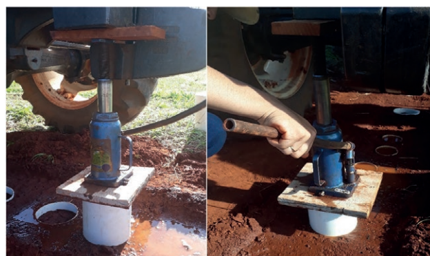
Fig. 1. Process of inserting the microlysimeter into the soil and collecting the soil to manufacture the microlysimeter with undisturbed soil.
