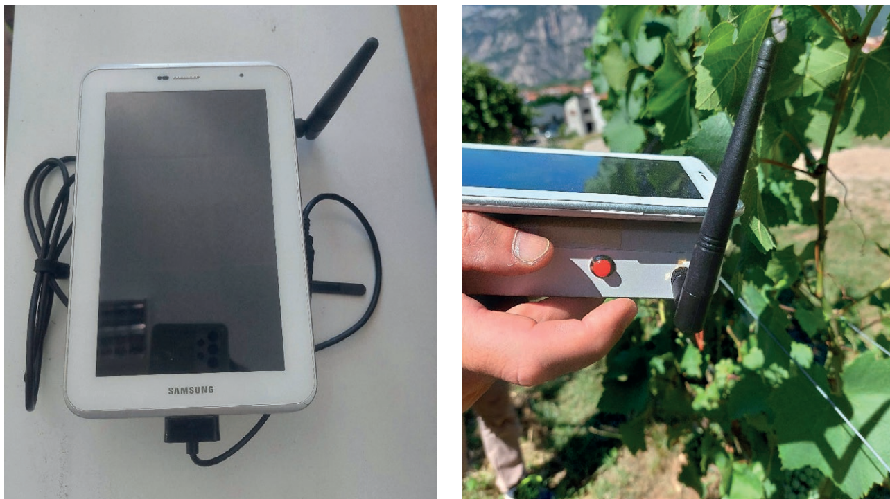
Figure 3. (a) Setup of CWSI slave station. (b) CWSI slave station measurements.
