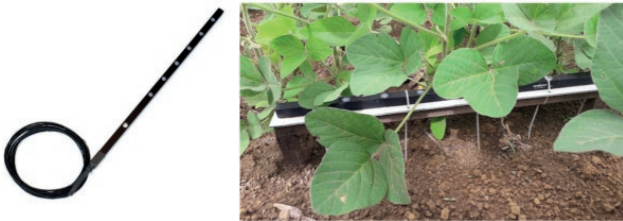
Figure 2. The PAR Apogee® SQ-316-S bar sensor (Apogee Instruments, Inc., Logan, Utah, USA) installed on the cultivation line of 75I77 RSF IPRO (ULTRA) cultivar in an experimental area at the Faculdade Marechal Rondon, in Vilhena, RO, Brazil (2018).
