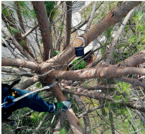
**Fig. 2.** Receiver position on the tree.
