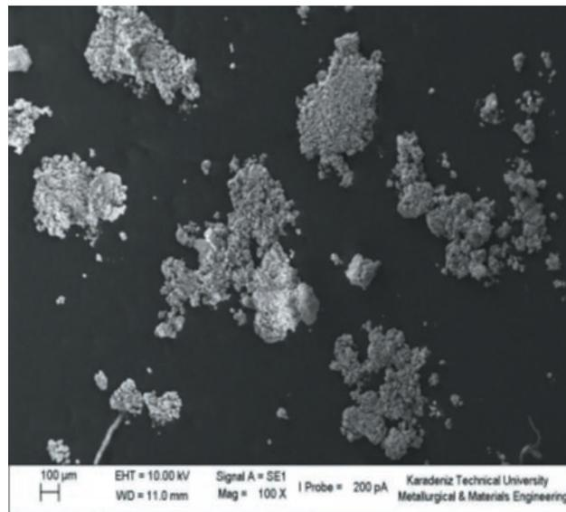
Figure 1. SEM images of ZnOTiO<sub>2</sub>NPs in dry form.
