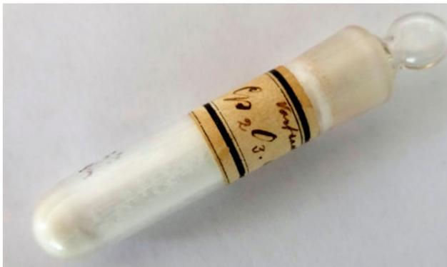
Figure 11. Test tube with a lutetium preparation (Cp<sub>2</sub>O<sub>3</sub>) originally produced by Carl Auer von Welsbach.
