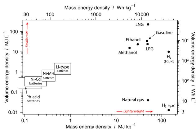
**Figure 4.** Volume and mass energy densities of some selected batteries and liquid fuels. Both MJ and Wh are reported in the diagram as energy units (on opposite sides), as both are largely diffused in the literature and technical documents.
