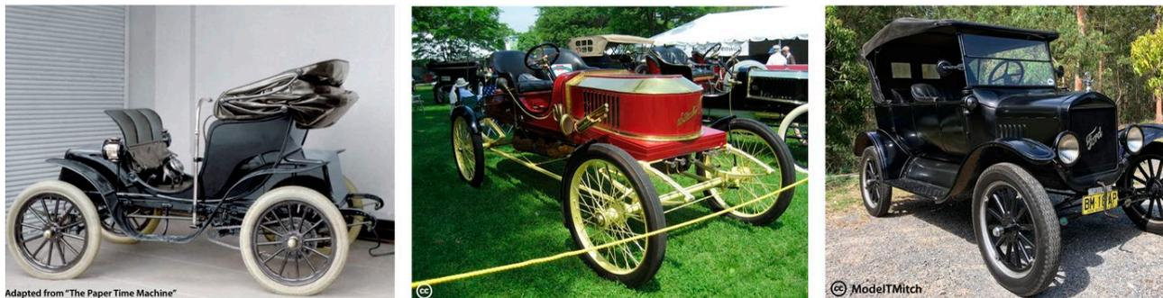
**Figure 1.** From left to right, examples of electric, steam and internal combustion engine cars of the early 20th century (1906, 1908, 1925, respectively).
