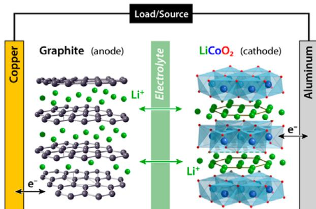
**Figure 5.** Scheme of a lithium ion battery, where  $\text{Co}^{4+}/\text{Co}^{3+}$  half reaction occurs at the cathode and redox-promoted intercalation of lithium in graphite takes place at the anode.
