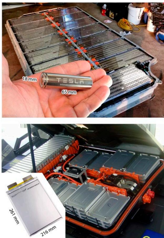
**Figure 6.** Individual cells for BEVs and their final assembly in the pack: Tesla (cylindrical, top) and Nissan Leaf (pouch, bottom).
