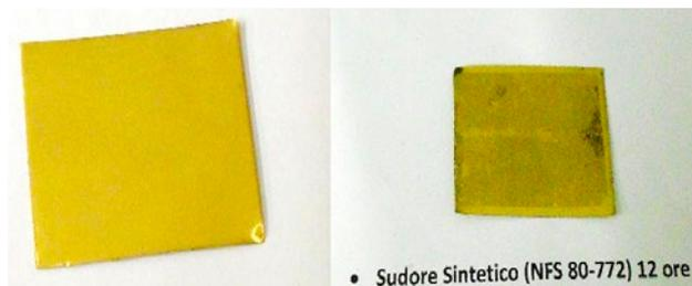
**Figure 5.** Corrosion test of a gold-plated sample, before (left) and after (right) 12 hours under syntenic sweat test.
