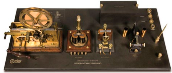
Figure 5. Radio receiver built in 1923 according to the model of Marconi’s receiver dating back to 1895. 4 A part from the battery box, all the other components like the coherer (right lower part, near to the antenna) are original.
