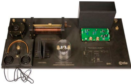
Figure 4. Radio receiver built in 1912, the model of it is in the booklet Father Alfani dedicated to Marconi during his visit held in 1912. 4 The diode, head-phones and the capacitor are original.
