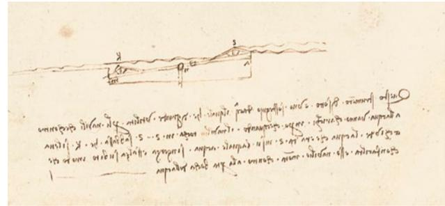
**Figure 28.** C.A., fol. 127v, detail: rocker water support.
