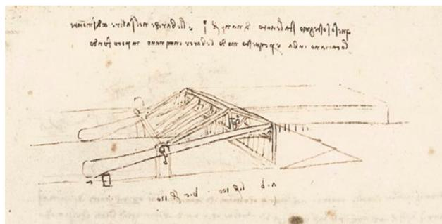
**Figure 26.** C.A., fol. 127v, detail: counterweight water support.
