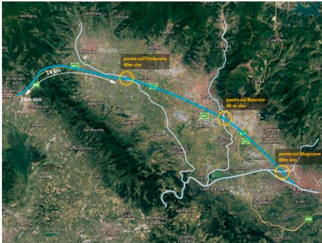
Figure 16. Satellite view of the plain between Florence and Pistoia with the route of the canal and the crossing of the tributaries of the Arno.
