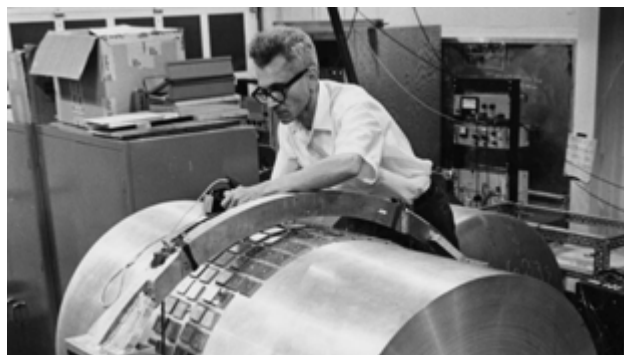
Figure 1. Weber's bar detector. Joseph Weber with his bar detector. The small metallic squares on the aluminum cylinder (the bar) are the piezoelectric crystals that were used to quantify the bar deformation. Image credit: University of Maryland Libraries Special Collections and University Archives.
