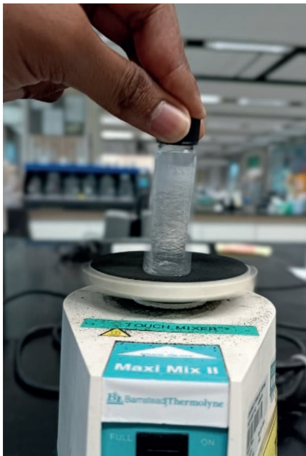
Figure 5. Preparation of demulsifier DB using Barnstead Thermolyne Maxi Mix II Vortex Mixer.
