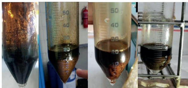
Figure 3. Test matrix of non-EOR demulsification test.
