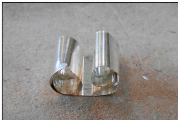
Figure 2. Cornet (top) and volute shapes (bottom) in the same rolled cupellation bead.
