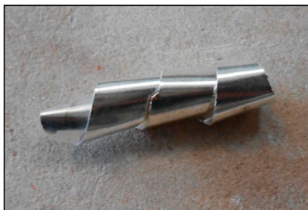
Figure 1. Characteristic gold parting steps on a laboratory scale. After the inquartation stage (a), the precious metal bead is hammered (b), rolled (c) and annealed (d). The parting process occurs inside a Kjeldahl flask (e), keeping the rolled specimen in a boiling acid solution (f).
