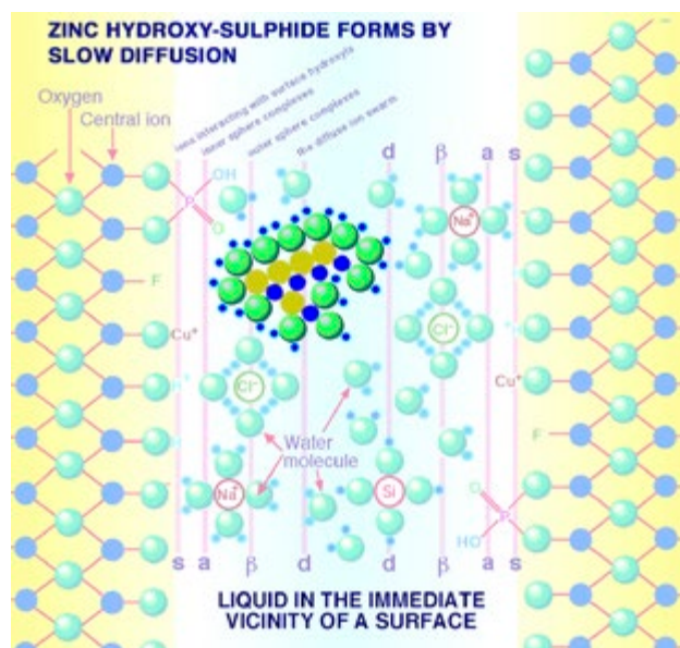
Figure 75. The initial solid phase of zinc sulphide precipitate is too small to be seen by SEM. In this diagram it is depicted as a hydrated nucleus surrounded by adsorbed water molecules. The oxygen atoms in this surface water are two hydrogen atoms short of those required to hydrate the cluster entirely with water molecules. The actual atomic geometry and hydration of a molecular cluster of this nature is quite difficult to determine and it is probably variable. It is quite important that some of the water molecules are dissociated. Hydroxyl groups have reacted with some or all of the high-energy lattice sites.
