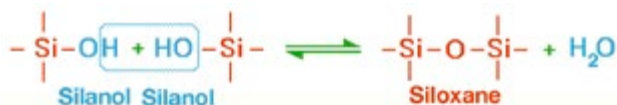
Figure 46. The basic reaction by which hydrated silica polymerises is divestment of water to form siloxane linkages.
