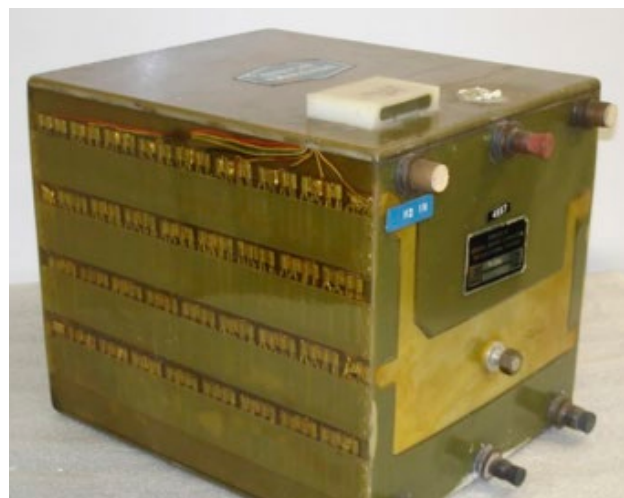
Figure 7. Sample Union Carbide KOH fuel cell for General Motors “Electrovan.” NMAH catalog no. 2007.3061.01. Smithsonian Image.
