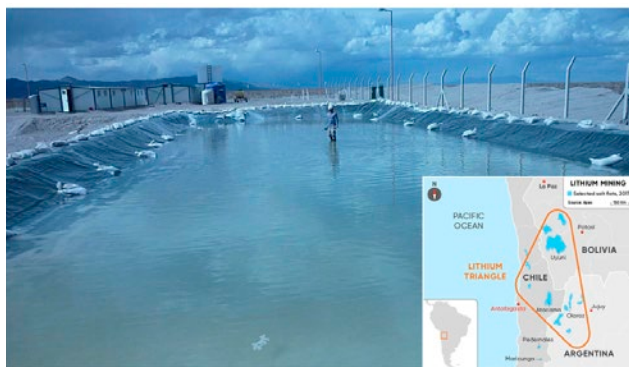
Figure 8. Lithium brine ponds in the Lithium Triangle, South America (bottom right map).
