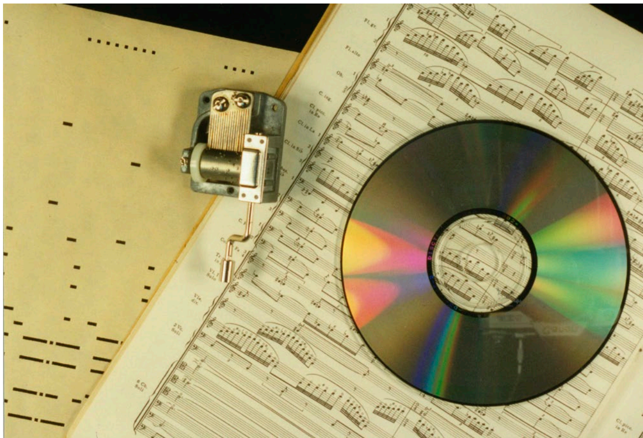
Figure 1. Four digital storage media. (a) The cylinder and comb from a music box play 16 bars from Lara's Theme (M. Jarre). The 18 tines of the comb have different masses and thus play different notes when struck by spikes on the cylinder. It has 18 parallel channels – circles round the cylinder. The loudness is binary (spike or no spike, note or no note). The timing is in principle analog, but is here quantised in multiples of 1/12 of a bar. The uncompressed data content of this cylinder is therefore 18 \times 12 \times 16 = 3456 bits. (b) The pianola roll in the background also has parallel binary channels, but the length of the hole determines the time the strings sound before the damper is replaced. In that sense, both duration and timing could be analogue, but again they are quantised in this example. The uncompressed data content is 35,000 bits per metre. (c) Standard Western music notation is (largely) parallel binary digital coding: each line and space (parallel channels) represents a pitch, though that pitch can be varied by sharps and flats. The time coding is encoded digitally in symbols (see Fig 2). This example ( The Rite of Spring , I. Stravinsky) has about 30,000 bits on this page, which lasts a few seconds, using a coding somewhat like that in Fig 2c. (d) The CD also carries a binary digital signal (“pit” or “no-pit” in the track) but it is different in all other aspects. The signal is carried in serial rather than in parallel, and it encodes numbers that are proportional to the pressure of a sound wave. This CD records about 5 \times 10^9 bits, not counting error correction bits. The storage efficiencies are approximately: a) 5 \times 10^5 bit.kg -1 , b) 10^6 bit.kg -1 , c) 10^7 bit.kg -1 , d) 3 \times 10^{11} bit.kg -1 . The apparatus required for re-creation varies greatly in size: that for (a) is shown ( \sim 0.01 kg), that for (c) is \sim 10^4 kg.
