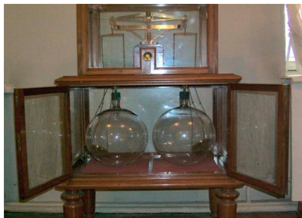
Figure 5. Mendeleev's Apparatus for Measuring Gas Densities. Photograph courtesy Roger Rea.
