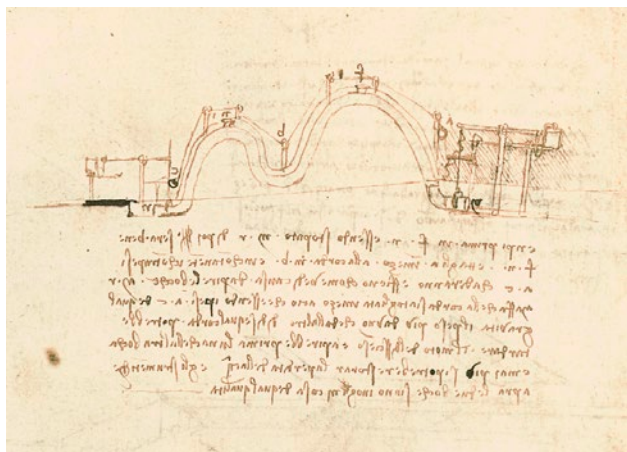
Figure 19. C.A., fol. 126r, detail: double siphon.
