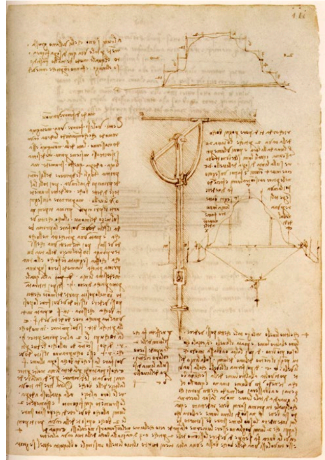
Figure 23. Codex Madrid I, c. 111r: level used to guide the excavation of a tunnel.
