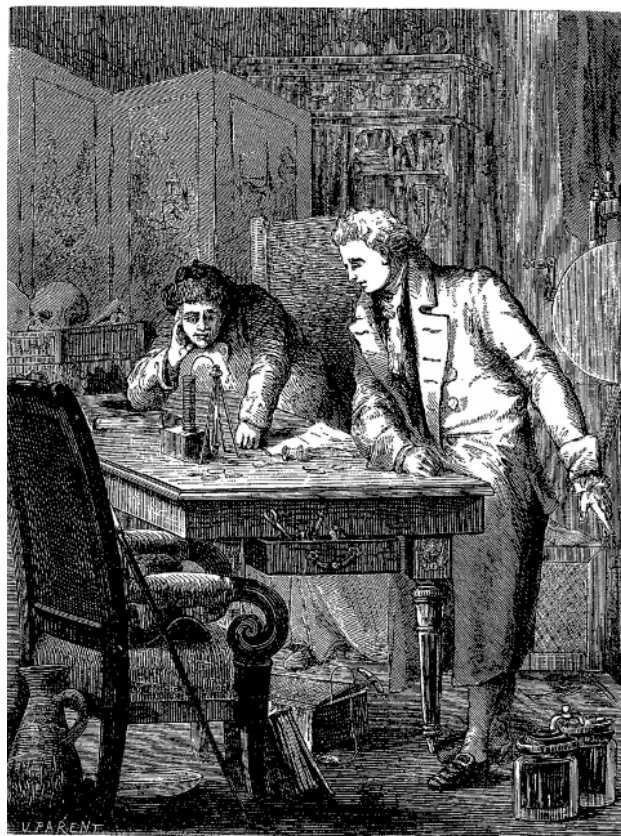
Figure 3. An illustration of an experiment of electrolysis by William Nicholson and Anthony Carlisle on May 2, 1800, by decomposing water by electricity of a Voltaic pile. Taken from ref. [45], “ La Pile de Volta ”, Chapter III, p. 629, Fig. 324.
