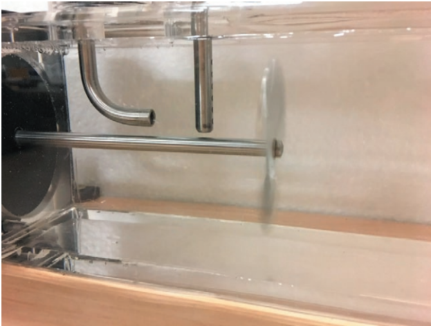
Figure 10. Cavitation completely prevented in gassed tap water after flowing 80% de-gassed water directly onto the rotating propeller blades (at 2300 rpm).
