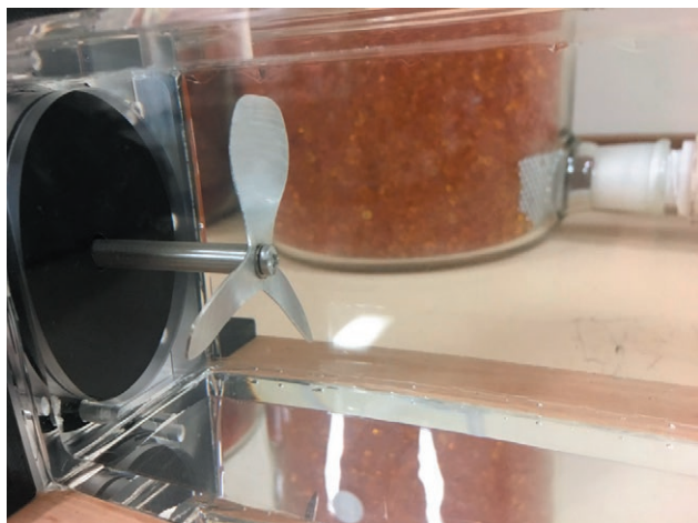
Figure 6. Photograph of the propeller used to study cavitation at the laboratory scale.
