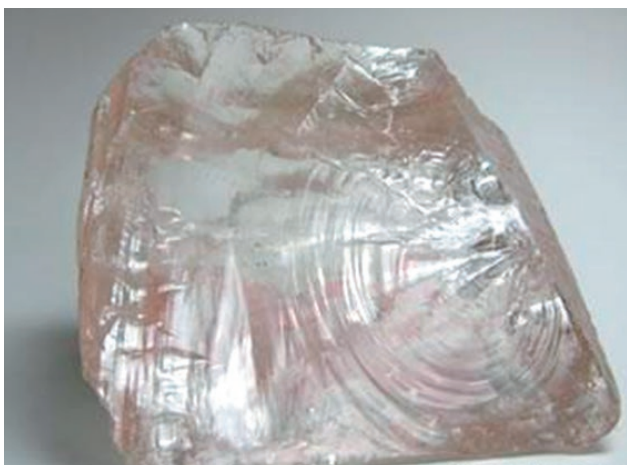
Fig. 11 Quartz: fracture surface ( https://geology.com/minerals/quartz.shtml ).
