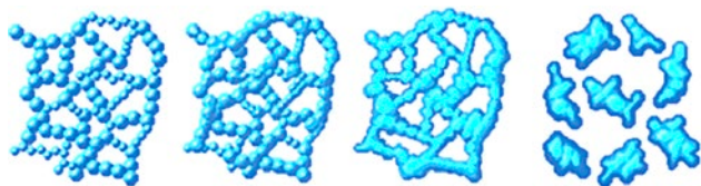
Figure 55. Stages in the aging of a gel are illustrated from the chaining of spheres and their greater coalescence, to the coarsened structure which results from drying or heating where the structure disintegrates to irregular rounded particles. [Adapted from Iler 2 , 1979, p. 530]
