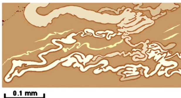
Figure 70. Ptygmatic micro-chert veins in a laminated matrix chert show the ‘loopy’ nature of the fluid precursor silica gel injected into a precursor ooze. Both matrix and ptygmatic veinlets are metacolloidal chert so the difference at the time the precursor was injected is in the gel structure or consistency - plastic gel and non-Newtonian fluid. The shear thinning property of the fluid silica polymer causes the looping and bulging. This specimen from Richie Lake 17 , Sokoman Iron-formation is illustrated by Dimroth and Chauvel (1973, p. 122).
