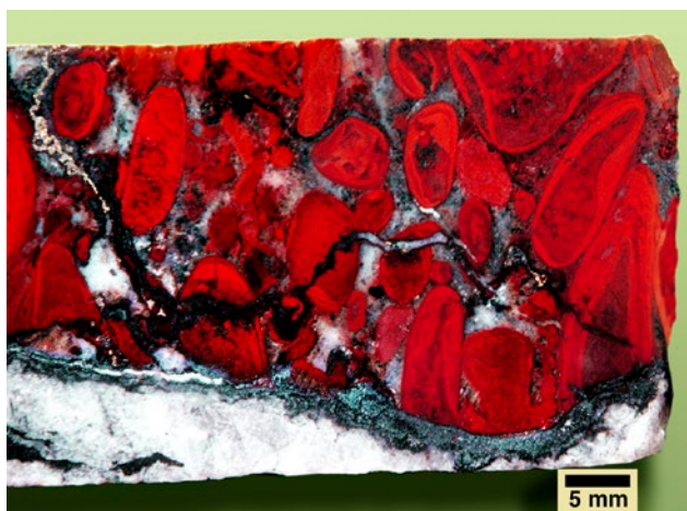
Figure 63. Brilliant jasper oolites occur in core through a quartz lode at the Abra Prospect, Jillawarra, W.A. Jasper is metacolloidal and a soft precursor stage of these overgrowths on accretionary siliceous nuclei is indicated by their plastic deformation, mutual indentation, and fragmentation. They are cut by later stylolitic quartz veinlets which meandered through the soft gelatinous silica precursors.
