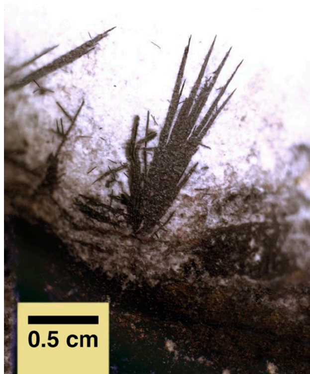
Figure 82. Radiating acicular hematite needles have grown out like spikes into a gelatinous dolomite precursor of the lode at Juno Mine, Tennant Creek. This 'wild growth' from a central nucleation point is typical of bladed and spherulitic crystal patterns developed in gelatinous media where enhanced (catalytic) crystal growth on one of the small seed crystal faces proceeds almost to the exclusion of growth on other faces.
