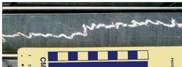
Figure 71. The detail of a ptygmatic quartz vein in the core of the New Cobar Mine at Cobar NSW, shows that it cuts across the cleavage yet it has been offset in places by further movement on the cleavage planes. Precursor polymeric vein silica also appears to have been mobile at this stage as small ‘spurs’ and offshoots of it project along the cleavage planes.
