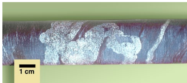
Figure 76. A ptygmatic-type clastic mud dyke or “dirty early quartz vein” has been intruded into soft diagenetic banded hematite shales. These early “out-wellings” of entrapped fluid through fine oozy sediment are episodic with each successive reactivation becoming more quartz rich until the filling material resembles vein quartz. Explorer 8 drill core, Tennant Creek.
