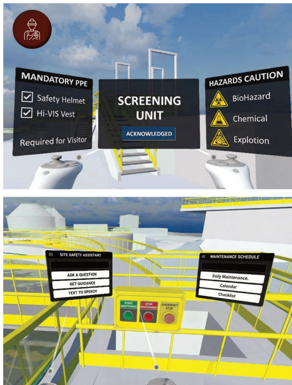
10 | Operator-profile interfaces showing support panels for operational procedures and maintenance tasks, integrated with AI-based guidance and reminders about the risks associated with each unit and the required PPE.
